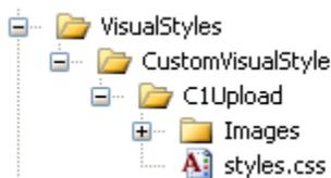
This structure of these folders is very important; **C1Upload** will always look for the `~/VisualStyles/StyleName/C1Upload/styles.css` path, as it is the default visual style path for the control.
